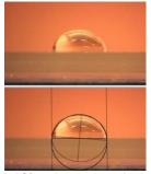
2.0% polymer on glass Oil contact angle: 82.0°
